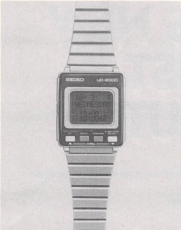
THIS IS NOT a wrist watch! It is the display module for the Seiko Datagraph computer.
